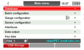
In the main menu, use the "↑" or "↓" keys to select a submenu, e.g. "gauge configuration", and confirm with the "OK" key to access the settings in this submenu.
