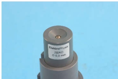
Zero calibration standard with inserted target ball
